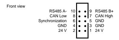
The ribbon cable connection is used to synchronize the detectors with each other and to provide the supply voltage and interface connection. The supply and interface connection to the control device can be made either using the ribbon cable or a plug terminal (see 6.1, Plug terminal: Supply and interface).
